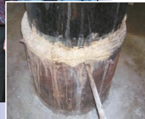
Home-made boiler to provide humidity and a constant temperature to the mushroom project
